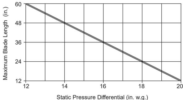
This damper's design at a blade length of 60" has a maximum allowable blade deflection of L / 360 for the static pressure indicated on the chart. At reduced blade lengths, higher static pressure limits can be attained without sacrificing damper operating performance characteristics.
